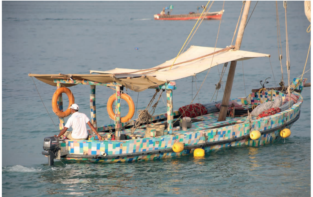
The 'Flipflop' boat as it arrived at the Zanzibar port having sailed 500km from Lamu, Kenya. The boat is made entirely of recycled plastic and its name derives from the fact that roughly 30,000 recycled flip-flops were used in its construction. Photo | Zainul Mzige
