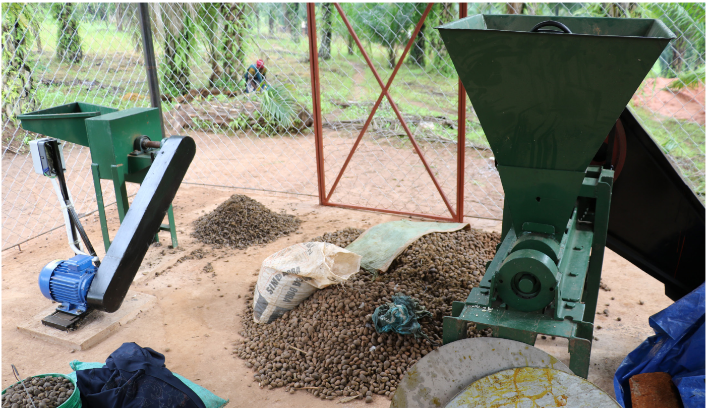
A photo of the machines used for grinding palm fruit into powder. Photo | UN Tanzania
